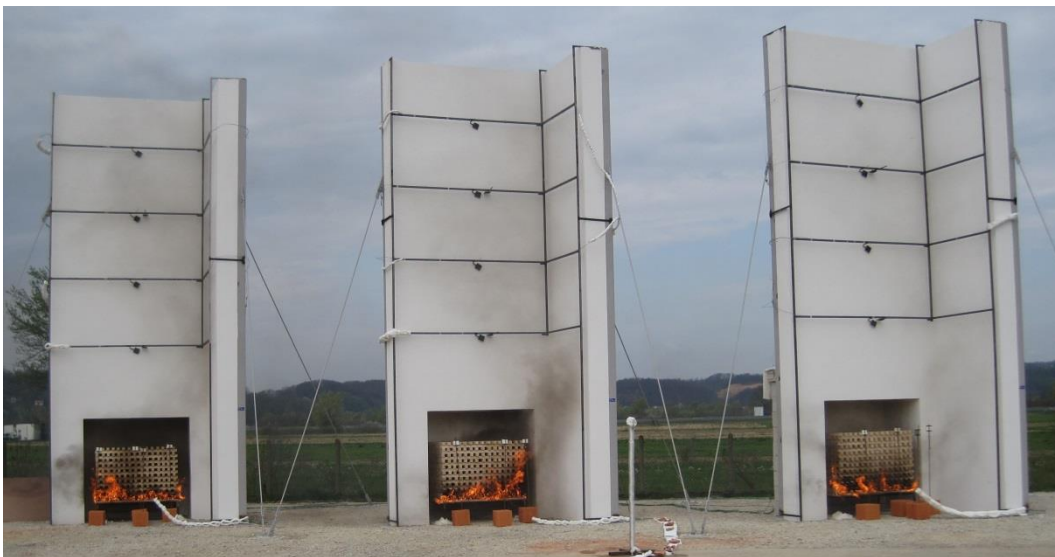
Figure 5. The three façades tested during the Zagreb tests in March.
