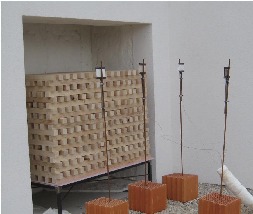
Figure 7. Position of plate thermometers in front of the combustion chamber.
